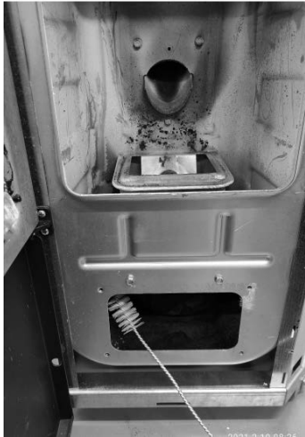
Fig. 61 - Clean with pipe cleaner
