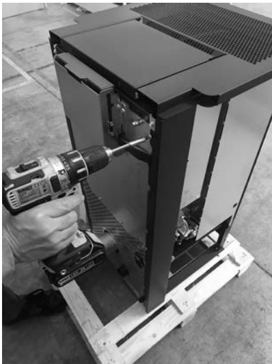
Fig. 35 - Remove the black profile
