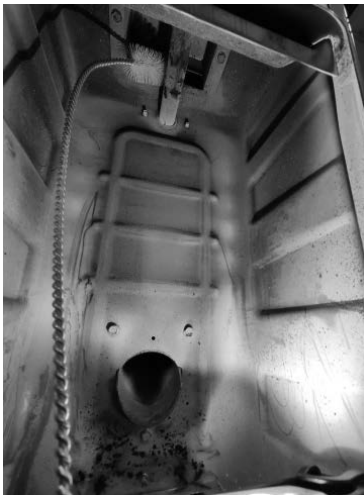
Fig. 63 - Clean with pipe cleaner
