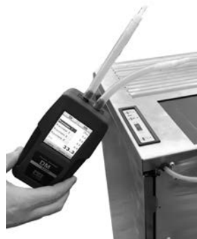
Fig. 54 - Digital pressure switch connection
