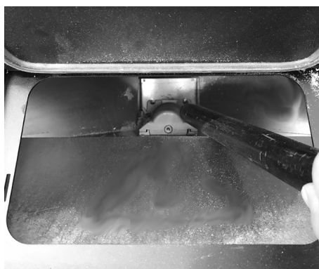
Fig. 26 - Hopper and auger cleaning
