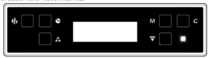
The control panel is managed by a microprocessor. The temperature detection system uses thermocouples. The large display improves the appliance management by making read-outs and functions promptly available. The main feature of the panel is the all-automatic management of the appliance. The controls and the various displays are described below.
