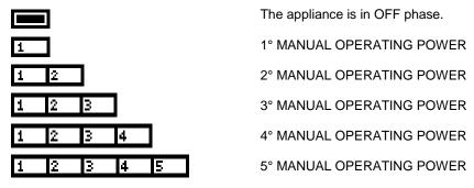
In this mode the user can choose to run the appliance from the minimum power (therefore with the minimum pellet consumption) to the maximum power (therefore with the maximum pellet consumption). In this case the appliance always runs at the set power without any modulation in accordance with the target temperature.
