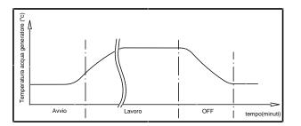
**WORK**: the duration depends on the ability of the system to receive heat. The generator's operating status is displayed. During this stage the brazier cleaning mechanism "Pellet Power", that is, the device installed inside the brazier, moves in timed mode.
