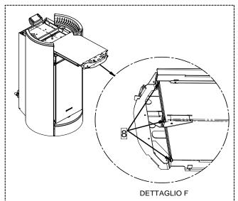
7 – Remove the pellet loading tray and loosen the 3 screws (8) underneath as shown in the detail.
