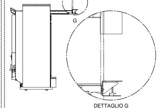
7 – Remove the pellet loading tray and loosen the 3 screws (8) underneath as shown in the detail.
