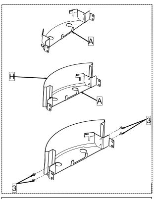
2- Take the lower bracket (A) supplied with the kit and fix the calendered profile (H) with the 4 screws (3) provided in the kit.
