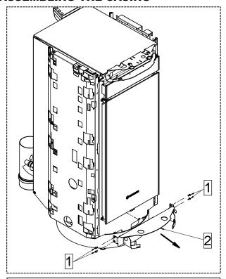
1- Undo the 4 screws (1) and remove the lower bracket (2) present on the appliance and dispose of it.
