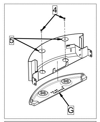
3 – Fix the lower cast iron element (G) to the lower bracket (A) just assembled, using the 2 screws (4) and the 2 washers (5).
