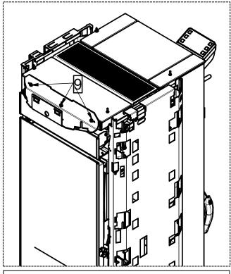
$9-\mbox{Loosen}$  the 3 screws (9) present at the top of the appliance.
