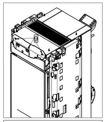
9 – Loosen the 3 screws (9) present at the top of the appliance.
