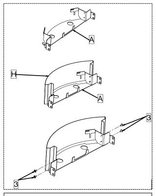
$2-{\sf Take}$  the lower bracket (A) supplied with the kit and fix the calendered profile (H) with the 4 screws (3) provided in the kit.
