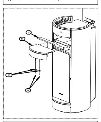
11 – Fix the cast-iron oven surface (M) using screws (9) and washers (10) as indicated in the figure. Install the non-structural profile (N) (only for model PAIRPLUS 13). **ATTENTION:** Carry out this operation only for air appliances.
