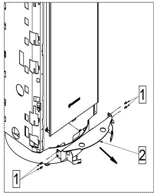
1- Undo the 4 screws (1) and remove the lower bracket (2) present on the appliance and dispose of it.
